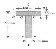
(b) Find the moment of inertia about the centroidal X-X and Y-Y axes of the angle section shown in figure.
