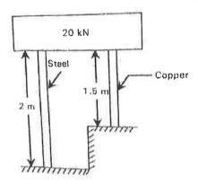
Diameter of each rod is 20 mm. Find the stresses in each rods. Take Es =  $2.05 \times 10^5$
